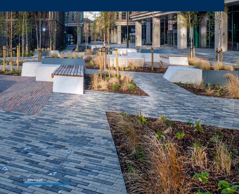
In total, around 480 bespoke elements, including bench units, seating steps, slabs and copings, were produced, weighing over 73 tonnes. Each piece was cast in a bespoke Granite White concrete mix, finished with a light acid-etch to achieve a clean, durable surface with subtle texture.
