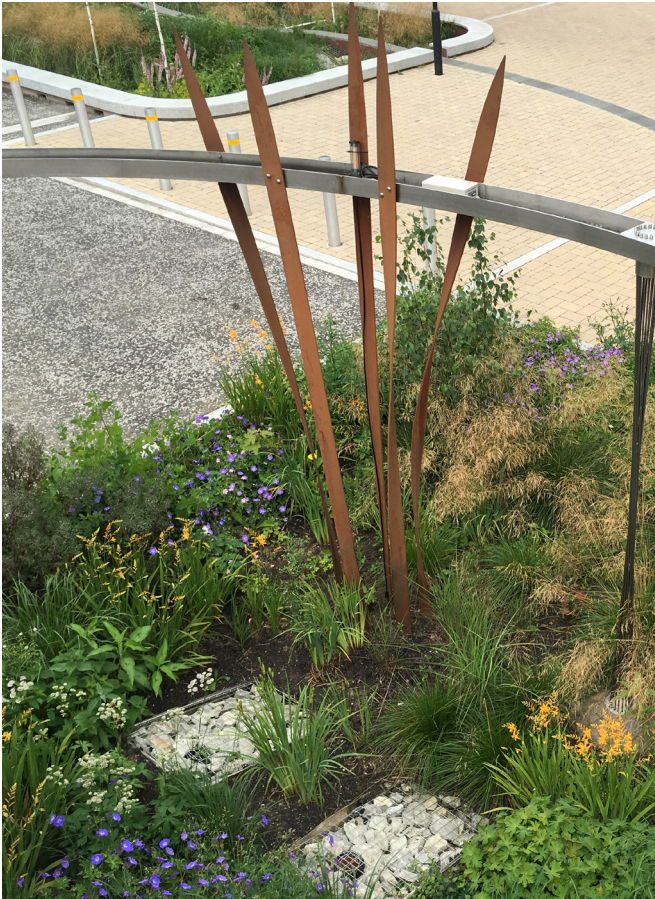
The original road surface has been replaced with attractive, 'self-draining' concrete block permeable paving. Clean water from the permeable paving passes into the planted basins. The 'wiggly wall' feature meanders through both paving and planting.
