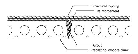
• Prestressed hollowcore slabs will exhibit a degree of camber, the extent of which will depend upon the span and the amount of prestress within the design. Due allowance must therefore be made for this in determining finishes and the overall floor thickness. The specified thickness of structural topping must be provided at the point of maximum camber.
