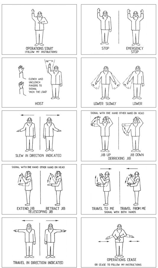
**Figure 6.8** Recommended crane signals
