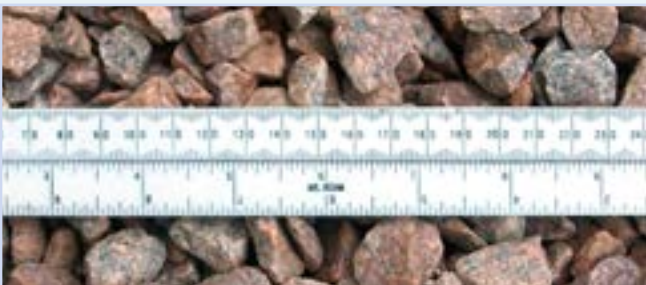
Permeable Aggregate – see above.
