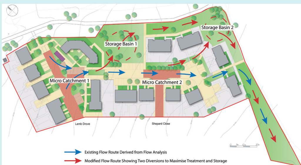
Two Micro Catchments gather and store water before it passes through additional SuDS features to Storage Basins situated along a new modified flow route.
